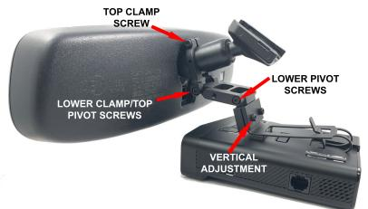
6 - Install the RD onto the mount. Make the necessary adjustments as shown above. Using the vertical adjustment and pivoting the Center Link, we recommend you adjust the RD as close to the bottom of the mirror as possible. If you are unable to get your finger between the RD and the mirror to access the top RD buttons, the spring clip is designed to be pushed downward to allow access to the top RD buttons as shown below in step 8.
